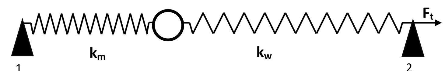
Fig.3 Physical model of strainmeter
